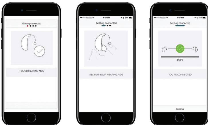
The app will populate with the data as programmed by your Audiologist and is ready to use. Pairing only needs to be done once, the devices will automatically reconnect when turned on and in range of the active Smart device.
