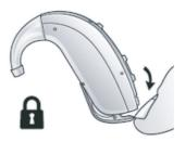
Insert tool straight into battery door lock.
