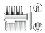
Insert the removal tip of the tool into the used wax guard so that the end of the tool touches the rim of the wax guard.
