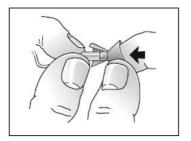
Check that the dome is securely in place by carefully lifting the lower part of the dome and verifying that the dome completely covers the end of the slim tube or receiver.
