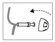
Push the new dome onto the slim tube or receiver firmly.
