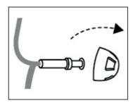
Remove the used dome by pulling it off the end of the slim tube or receiver.
