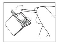
1. Removing the old microphone filter
