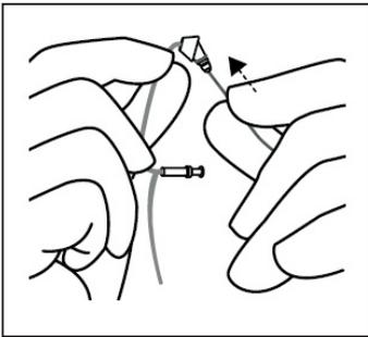
2. Now, push the cleaning wire through the top of the slim tube where it connects to the hearing aid. Thread the cleaning wire completely through to fully remove any debris.
