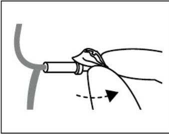
4. Check that the dome is secure by carefully lifting the lower part of the dome, and verifying that the collar completely covers the ribbed end of the slim tube.
