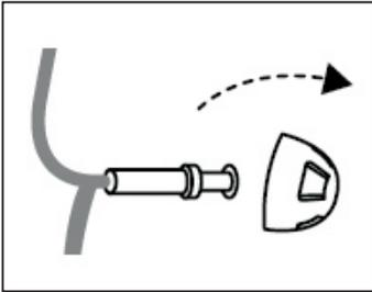
1. Next, remove the dome by pulling it off the ribbed end.
