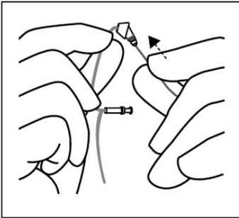
5. Finally, push the slim tube back onto the hearing aid until it clicks firmly in place.
