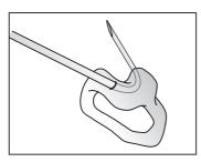
4. Pull the pointed end of the tubing through the earmould until the other end of the tubing is vertical and sits flat against the mould.
