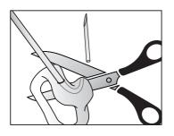
5. Cut off the pointed end as close to the earmould as possible. Ensure there no rough edges of the tube left sticking out as this can cause irritation in your ear.
