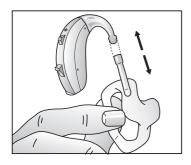
1. Remove your earmould from your hearing aid and then pull the tubing from the earmould.
