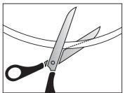
2. Cut approximately the last 5cm of pre-bent piece of tubing to a tapered end.
