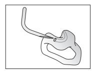
3. Feed the pointed end through the hole in the earmould from the outside as shown, until it emerges at the other end. If you have two holes in your earmould push the tubing through the bigger hole at the top.
