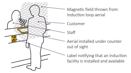
Below is a diagram of a room hearing loop (e.g. at an event, place of worship etc)
