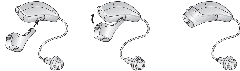
Attaching the DAI click-on adapter to Ambio, model 62.
